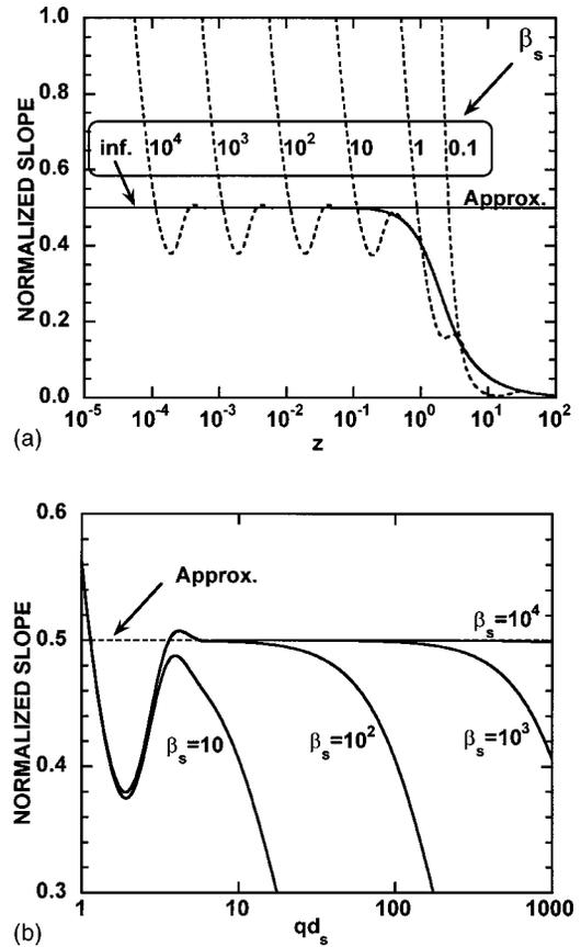
FIG. 1. Normalized slope [Eq. (8)], compared to the approximate normalized slope of 0.5, is shown for different  $\beta_s$  values: (a) as a function of the nondimensional parameter  $z$ , and (b) as a function of the nondimensional parameter  $qd_s$ . The line source and semi-infinite substrate approximations can be used with less than 1% error if  $z < 0.2$  and  $qd_s > 5$ .
