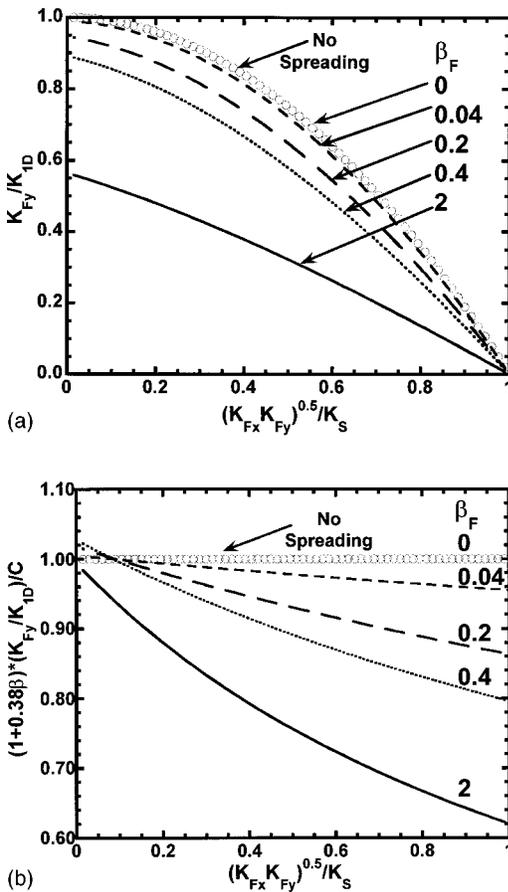
FIG. 3. (a) Ratio of the true thermal conductivity of the film to the one-dimensional thermal conductivity, and (b) the ratio from (a) normalized to  $C/(1+0.38\beta_F)$ , as a function of thermal conductivity contrast between the film and substrate.
