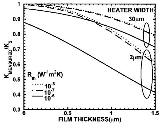
FIG. 8. Ratio between the thermal conductivity of the substrate as determined from the slope method for a film-on-substrate system, and the true substrate thermal conductivity, plotted as a function of the film thickness. The calculations are carried out for 2 and 30  $\mu\text{m}$  wide gold heaters of 2000  $\text{\AA}$  in thickness, deposited on a  $\text{SiO}_2$  film on Si-substrate system with different thermal boundary resistances between the heater and the film.
