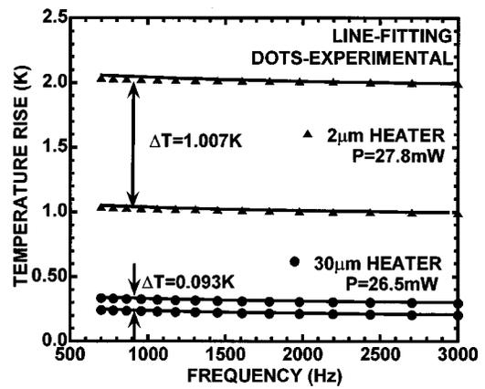
FIG. 6. Experimental temperature rise (dots) measured by 30 and 2  $\mu\text{m}$  width heaters deposited on the Ge-quantum-dot-superlattice and the reference samples. The experimental signal is compared to predictions for the temperature rise of the heaters (lines) calculated based on Eq. (1) for the fitted values of the in-plane and cross-plane thermal conductivity of the film.
