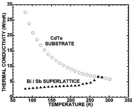
FIG. 4. Experimental thermal conductivity of a Bi/Sb superlattice and the CdTe substrate. The substrate thermal conductivity is comparable to the superlattice thermal conductivity at the upper end of the temperature range and a significant film/substrate thermal conductivity contrast effect is expected for this temperature range.
