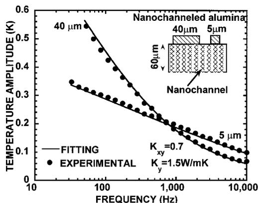
FIG. 2. Experimental temperature rise (dots) and the fitting based on a two-dimensional heat conduction model (lines) for a nanochanneled alumina sample (see inset for sample configuration) with anisotropic thermal conductivity. The experiment is carried out for two heater widths and the fitted values for the cross- and in-plane thermal conductivity are respectively  $k_{S_y} = 1.5$  W/mK and  $k_{S_x} = 1.05$  W/mK.
